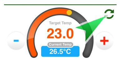
From here you can select a valve position instead of temperature. This is similar to how a manual TRV operates.
